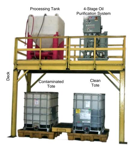
This System will process a 320 gallon tote in 1 to 3 days depending on the level of contamination.
