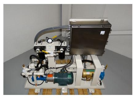
Prior to building this system IFS worked with the gearbox manufacturer to establish the flow rate, temperature requirements and oil quality required to maximize performance and gearbox life.
