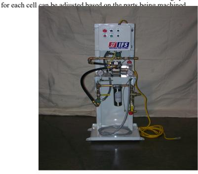
The final step in the project was the addition of auto makeup valve on each CNC machine. Operators now focus on machining and coolant levels in 200 gallon sumps are maintained within 5 gallons. Data collected has shown coolant temperatures and concentrations are very consistent.
